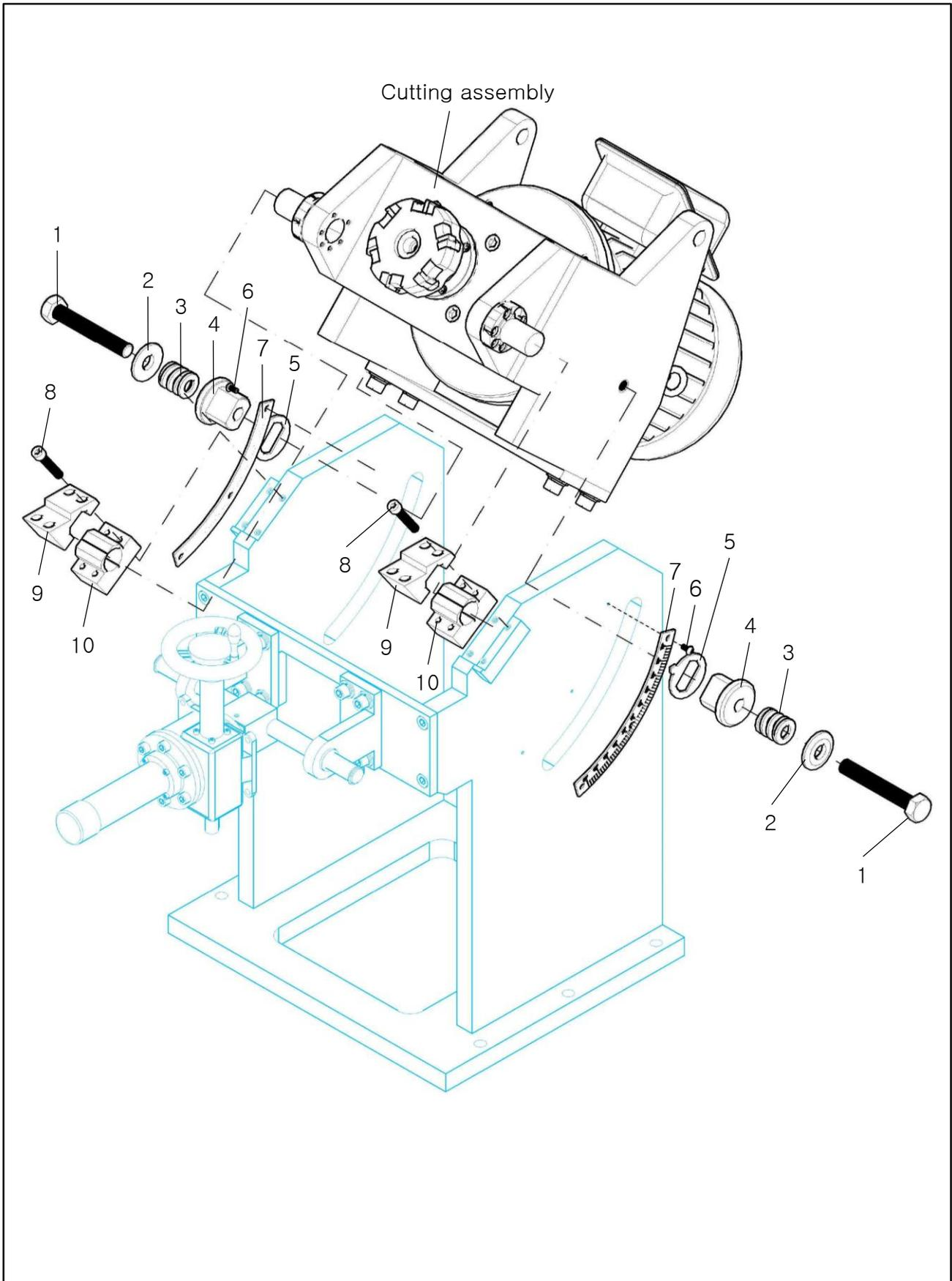
CUTTING ANGLE ADJUSTMENT PART-2 ASSEMBLY PARTS LIST
